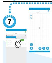
Tap **Identify** next to a device in the device list to make a device blink. Once you have correctly identified a device, tap the arrow next to identify and tap a space to place it on the grid.
