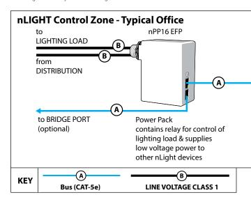
**CAT5e Writing Steps** (Note: Assuming all line voltage/dimming wiring completed)
